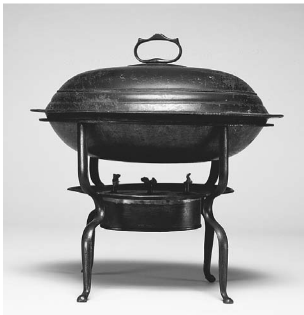
Food is often prepared at the table, as in the case of this curious old implement called Passmore’s Patent Conjurer made by Thomas Passmore of Philadelphia, circa 1797. Constructed of sheet iron and wrought iron, the conjurer permitted small articles of food such as oysters or lamb chops to be cooked over oil lamps in the manner of a pressure cooker. ROUGHWOOD COLLECTION. PHOTO CHEW & COMPANY.
